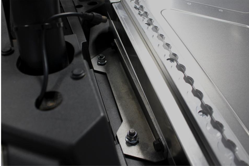
5. Using an 8mm Hex key to hold the position on the bottom side of the fastener system and a 15mm socket on the top nut, tighten the bracket down so it still has some adjustability.
