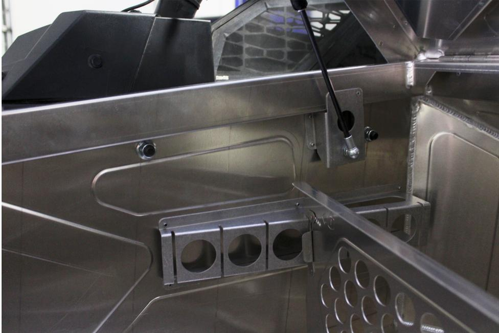
7. Finish the install by completely tightening the mounting bracket to the bed pan, again using the 15mm socket and the 8mm kex key.
