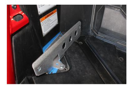
6. Remove the Driver Side mounting bracket. Use a 5/16" drill bit to drill the three mounting holes you marked in step 5
