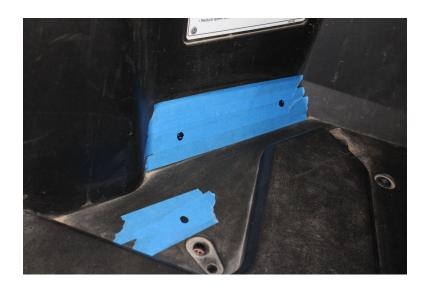
7. Place Aluminum Washer,SM in forward rectangle mounting hole recess See BOM, Item 9
