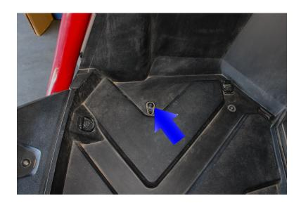
5. Use 2 of the supplied 6mm bolts to hold the Driver Side mounting bracket in place. Mark the 3 remaining holes to be drilled.
