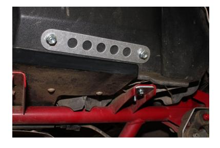
11. Install Aluminum Washer, LG and M6 lock nut.
